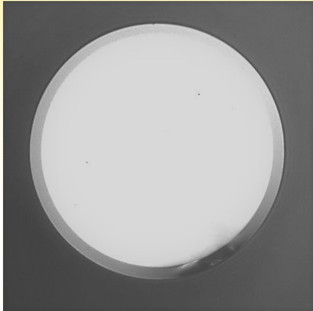
FIBER AT CONNECTOR END (PROXIMAL END) AFTER USE, AND STILL NO VISABLE DAMAGE
